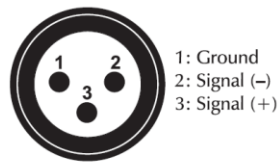
DMX-input XLR mounting-plug:
